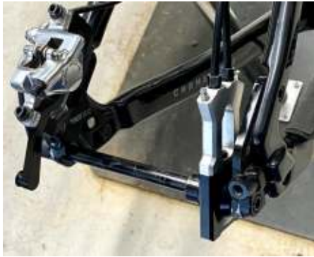
1.1: Remove the wheel and attach the actuator to the thru-axle or thru-bolt as shown.
