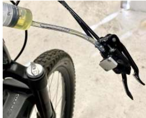
2.6: Observe the oil flow through the operator syringe.
