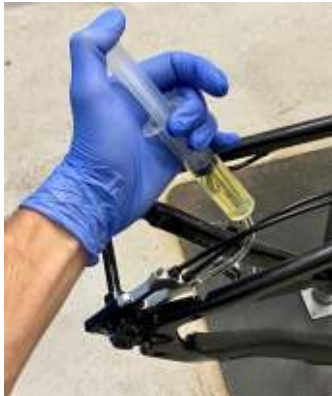
2.5: Push fluid from the actuator to the shifter. This will force any air bubbles into the reservoir, and then into the syringe.
