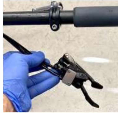
2.3: If not performed already, loosen the Onesie operator from the handlebar clamp.
