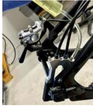
2.2: Attach a syringe with 30ml of mineral oil to the forward-facing nipple and open it using a 5 mm spanner
