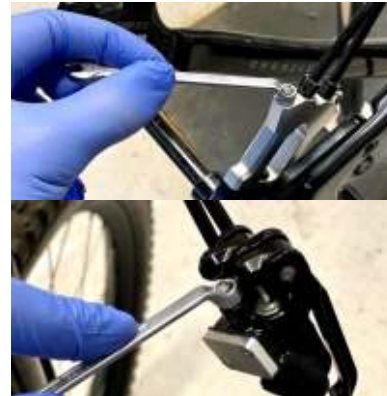
2.7: When no more air bubbles emerge in the operator syringe, close both nipples. Leave both syringes attached for step 3.
