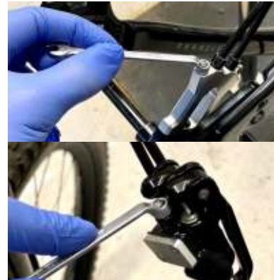
1.7: When no more air bubbles emerge in the operator syringe, close both nipples.
