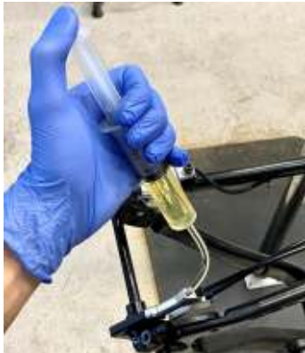
1.5: Push fluid from the actuator to the shifter. This will force any air bubbles into the reservoir, and then into the syringe.
