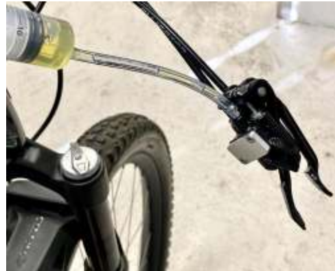
1.6: Observe the oil flow through the operator syringe.
