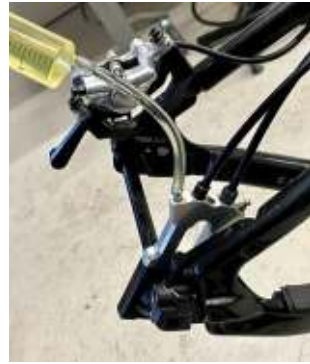
1.2: Attach a syringe with 30ml of mineral oil to the rear-facing nipple and open it using a 5 mm spanner
