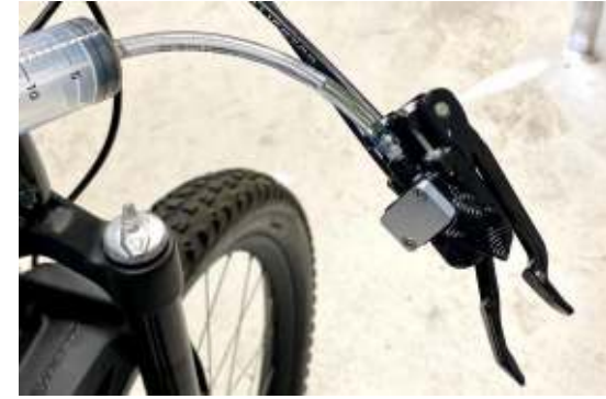
2.4: Open the shift lever nipple and attach an empty syringe, or a hose with a drain cup.
