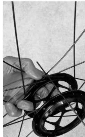
**Lacing:** Only tighten the nipples a few turns during lacing. This will make it easier to lace the remaining spokes.
