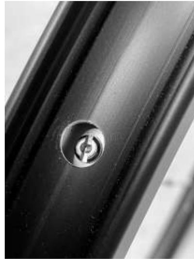
1.3: Tighten the nipple such that the spoke is flush with bottom of the nipple slot.
