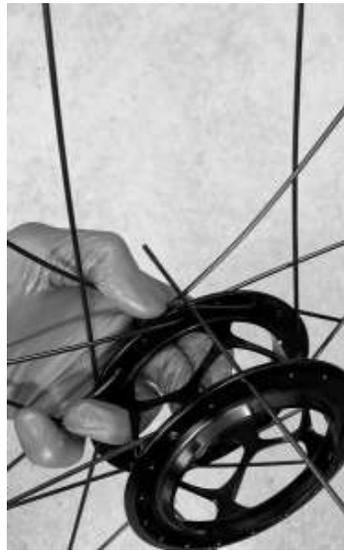
**3.2:** Carefully bend the NDS spokes down to pass through the DS trailing spoke.
