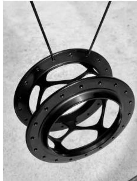
**1.2:** Pick the second next hole in the NDS flange and insert a spoke as in step 1.1.
