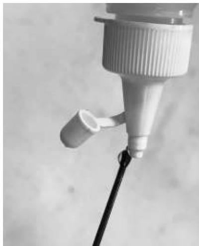
**Thread locker:** Using linseed oil will allow the nipples to rotate freely during tensioning, but seize up after a few days. This will reduce the likelihood of the nipples unwinding if the rim is damaged or bent.
