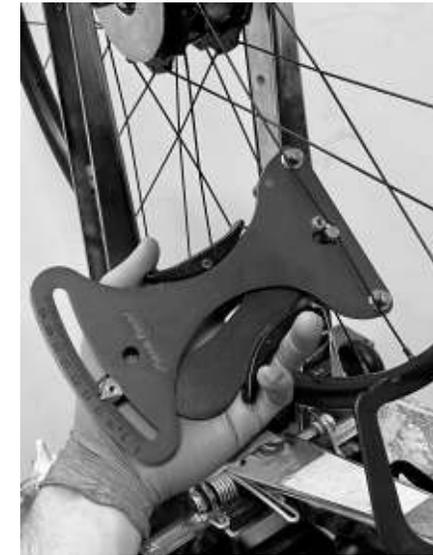
**Spoke tension:** Regularly check the spoke tension. An evenly tensioned wheel will require little truing and re-dishing afterwards.
