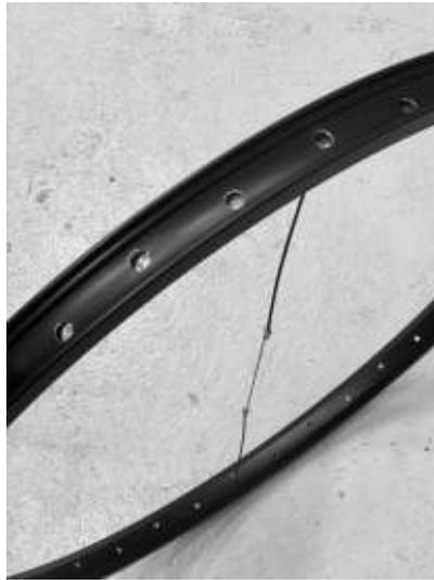
1.2: Install the spokes in two co-axial holes (180 deg. from each other).
