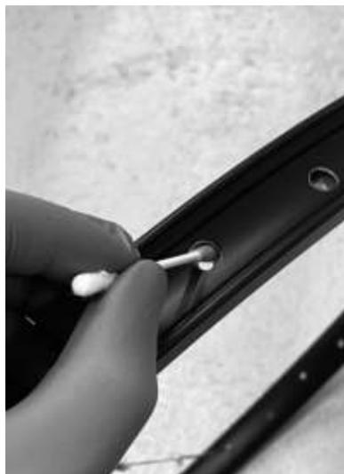
**Rimbed lubrication:** We recommend lubricating the rimbed slightly with Kindernay Velvet fluid, motor oil or other similar lubricant. This will allow the nipple to rotate more easily during tensioning.
