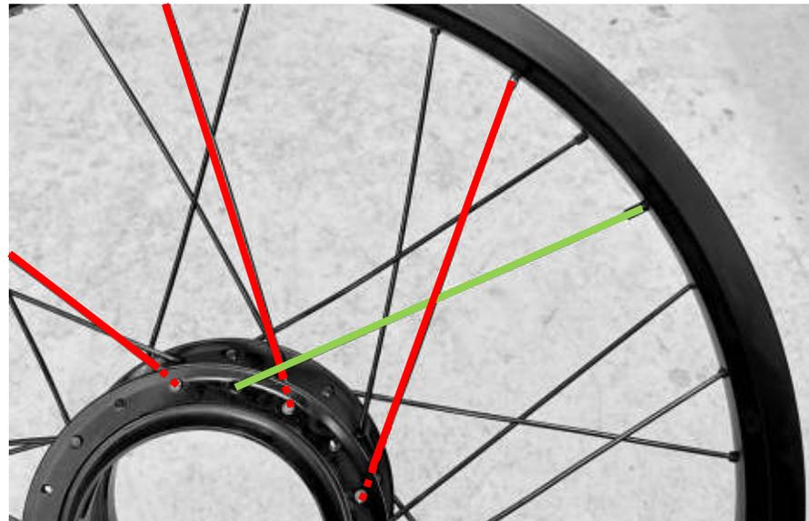
4.2: Route the spoke over the first trailing spoke, then under the last trailing spoke. The spoke should be routed as shown, with trailing spokes in red and leading spoke in green.
