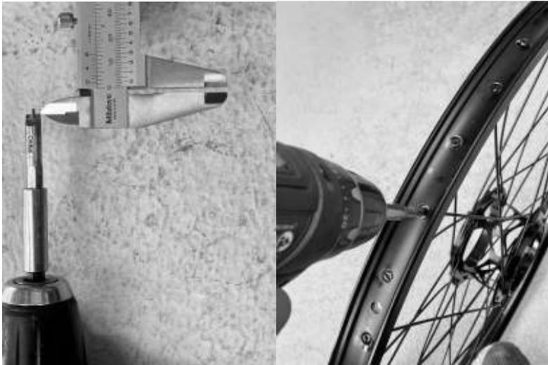
**5.1: (Optional)** Use a battery drill with a suitable spoke nipple bit to take up the initial slack. For most wheels, the limiter extension can be set to around 2 mm for the initial tensioning.
