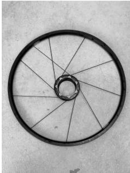
2.2: Route the spoke over the two first trailing spokes, and under the last trailing spokes.
