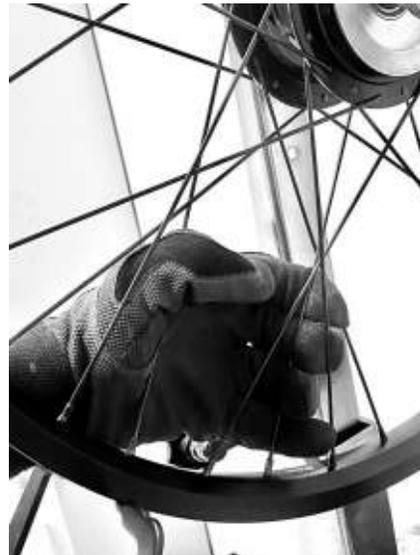
**De-stressing:** It is important to destress the spokes several times during tensioning. This will ensure the nipple and spoke are properly seated in the rim and SWAP cage, respectively.
