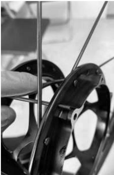
2.1: Install a spoke in any of the remaining NDS flange holes, exiting on the outside of the flange.
