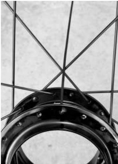
**3.1:** Insert a spoke in any drive side flange hole to the right of a NDS trailing spoke, exiting on the inside of the flange.
