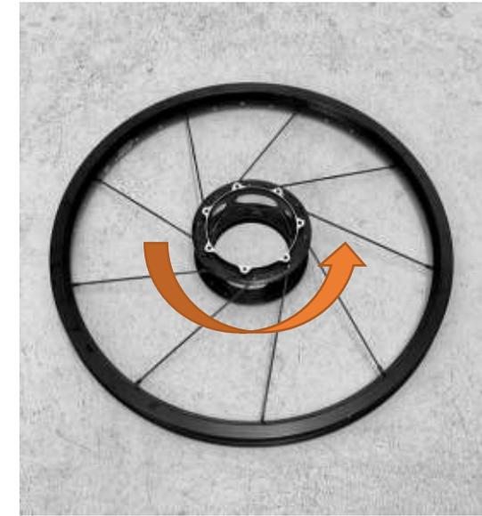
1.4: Complete the remaining spokes in a similar manner. Rotate the SWAP cage counter-clockwise, as seen from NDS to take up the initial slack.
