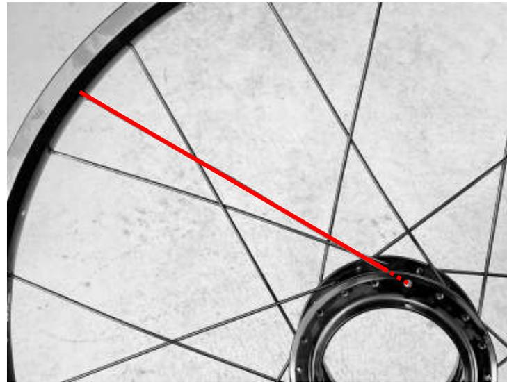
**3.3:** The spoke should be routed as shown in red, entering the rim to the right of the NDS trailing spoke referenced in step 3.1.
