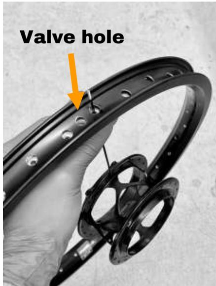
1.1: Insert a spoke in any of the non-drive side flange holes (the side with the threaded holes), exiting on the inside of the flange. Pass it through the spoke hole to the right of the valve hole.
