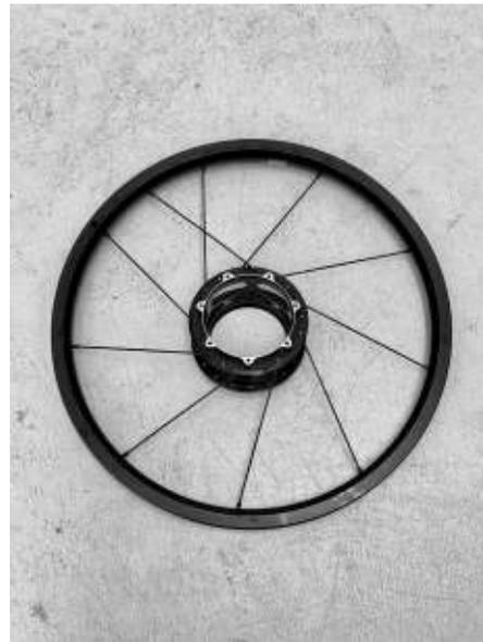
2.2: Route the spoke over the first trailing spoke, and under the last trailing spoke.
