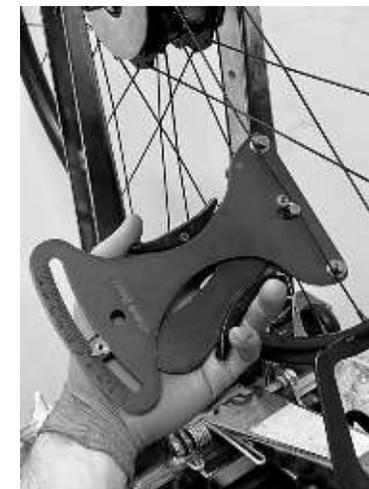
**Tensioning:** Ensure even spoke tensions to maximize the longevity of the wheel components.
