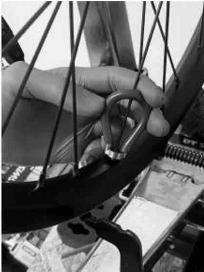
**Tensioning:** Be methodical in the tensioning process and pay attention to the spoke rotation to avoid spoke twist.
