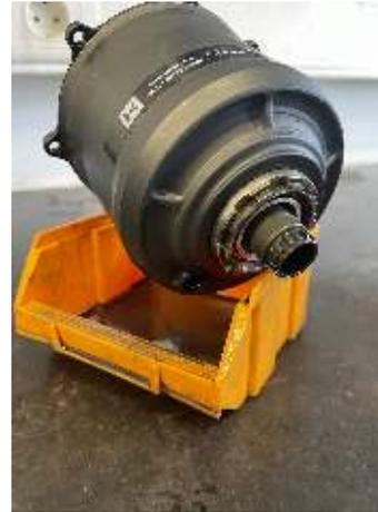
**1.3:** Allow gear hub to drain fully, approx. 5 minutes
