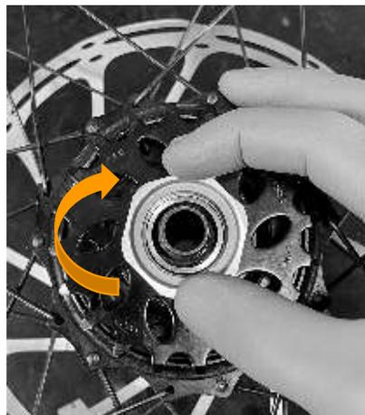
**4.2:** Install the hub sprocket locking by rotating clockwise.
