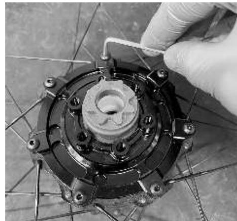
**1.3:** Install the gear hub in the SWAP, align the bolt holes and install the bolts.
