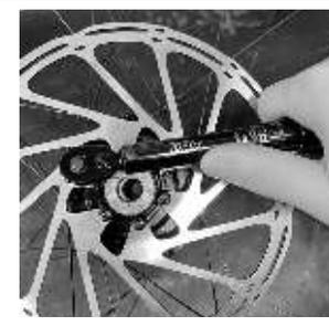
**2.3b:** Tighten the bolts to 6 Nm in a star pattern.
