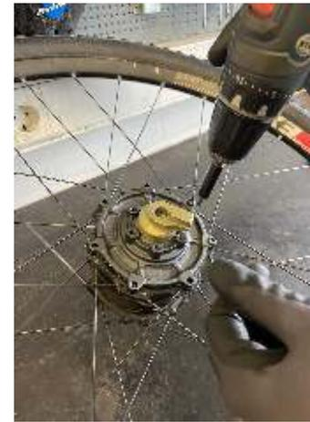
**1.4:** Remove gear hub mounting bolts
