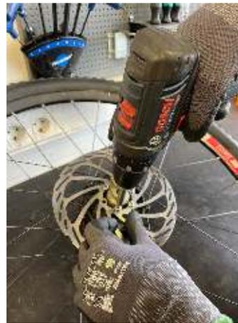
**1.3:** Remove brake rotor mounting bolts and rotor from hub
