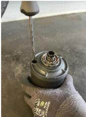
**1.1:** Remove oil plug from gear hub using T25 Torx Screwdriver
