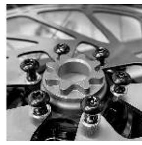
**2.2b:** Install the rotor bolts with the supplied bolts as shown.
