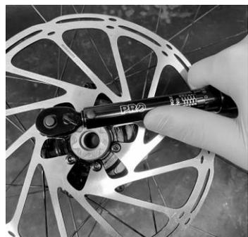
2.2a: Tighten the bolts to 6 Nm in a star pattern.
