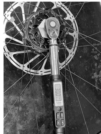
4.3: Torque the locking to 30 Nm.
