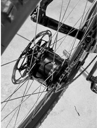
9.1: Install the chain/belt on the gearhub sprocket.
