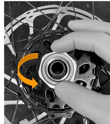
6.3: Remove the locking by rotating counterclockwise.
