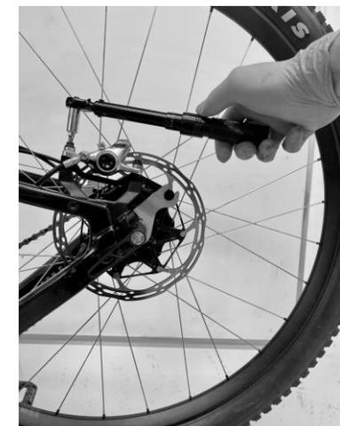
7.4: Torque the PM bolts to 9 Nm.
