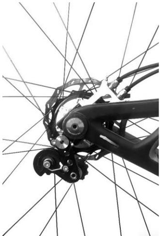
10.1: Mount the chain tensioner to the bike's original drop-out.
