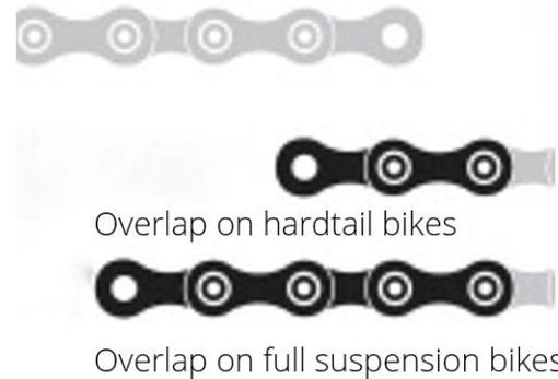
10.3: Wrap the chain around the front and rear sprocket. Add additional chain links according to you bike type.
