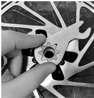
3.1: Install the torque arm.
