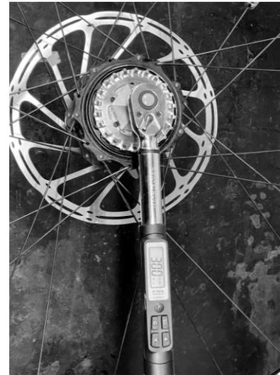
5.3: Torque the locking to 30 Nm.
