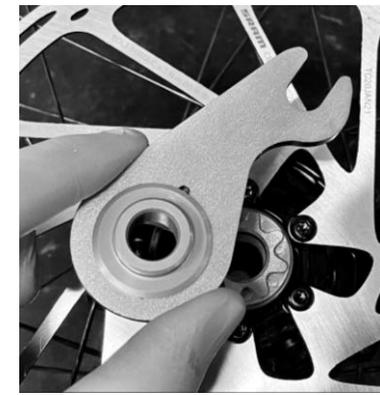
3.5: Remove the torque arm and match cap.
