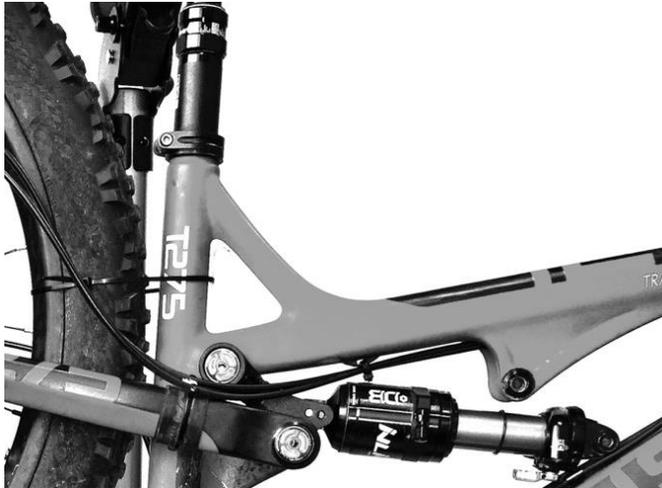
10.2: For full suspension bikes: Unbolt or let the air out of the shock. Zip-tie the rear triangle in the maximum travel position.
