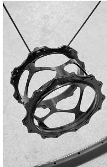
1.3: Pick the second next hole in the NDS flange and insert a spoke as in step 1.1.
