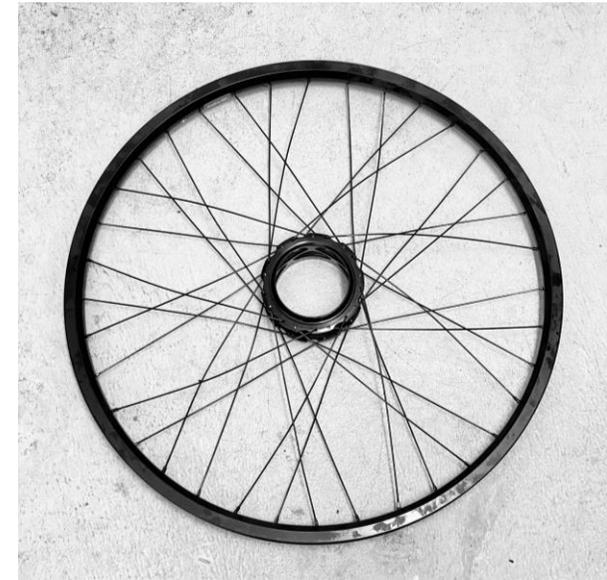
4.3: Repeat for the remaining spokes, completing the wheel lacing.
