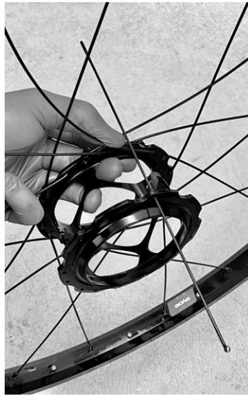
**3.2:** Carefully maneuver the DS spoke between the NDS spokes. It is ok to bend the spoke slightly in this process.
