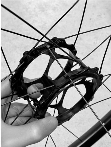
4.1: Install a spoke in any of the remaining DS flange holes, exiting on the outside of the flange.
