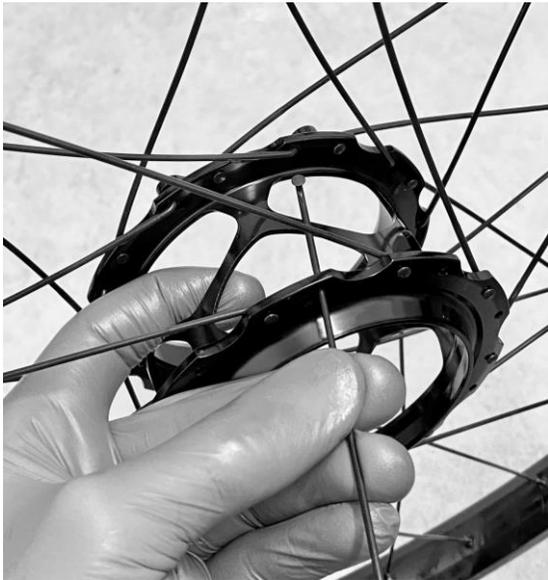
4.1: Install a spoke in any of the remaining DS flange holes, exiting on the outside of the flange.
