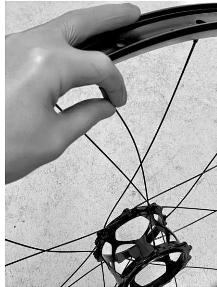
3.2: Carefully maneuver the DS spoke between the NDS spokes. It is ok to bend the spoke slightly in this process.
