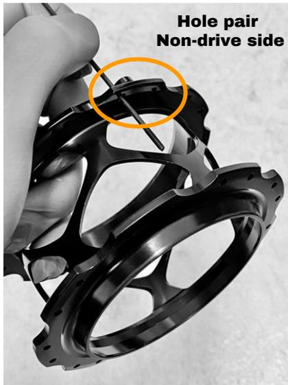
1.1: Insert a spoke in a non-drive side flange hole (the side with the threaded holes), through the left hole in the hole pair as seen from the drive side (as shown).
