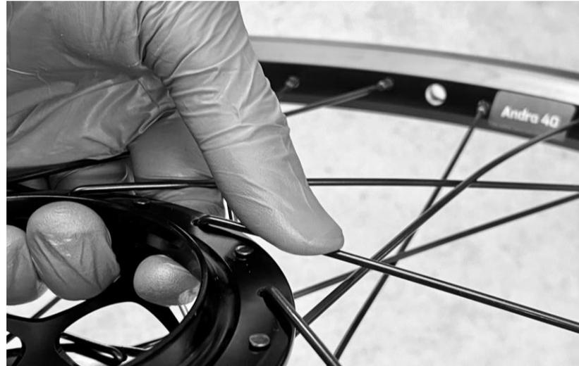
**5.2:** Align the leading spokes on NDS and DS flanges by pressing down on the spoke as shown. This is especially important for small wheels, as the large flange diameter gives large spoke angles. Otherwise, fatigue life will be reduced, and the spokes can loosen over time.
