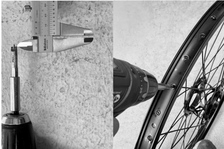
**5.1: (Optional)** Use a battery drill with a suitable spoke nipple bit to take up the initial slack. For most wheels, the limiter extension can be set to around 2-3 mm for the initial tensioning.
