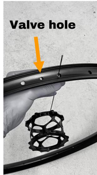
1.2: Pass the spoke through the spoke hole to the right of the valve hole.
