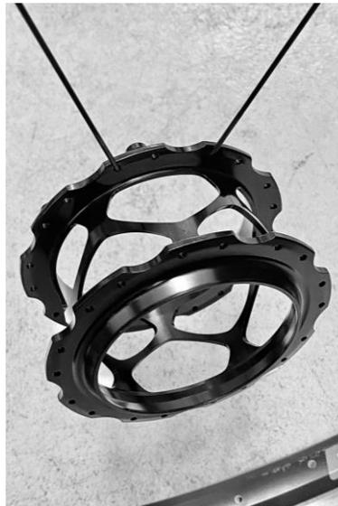
1.3: Pick the second hole next in the NDS flange and insert a spoke as in step 1.1.
