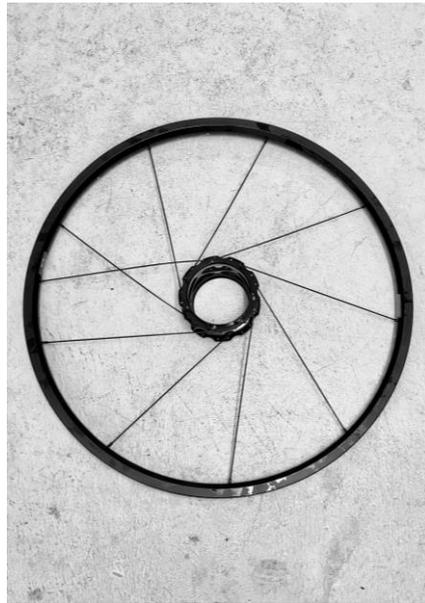
2.2: Route the spoke over the two first trailing spokes, and under the last trailing spokes.
