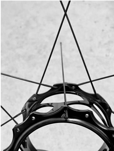
3.1: Insert a spoke in any drive side flange hole to the right of a NDS trailing spoke, exiting on the inside of the flange.
