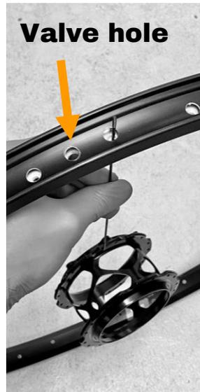
1.2: Pass the spoke through the spoke hole to the right of the valve hole.
