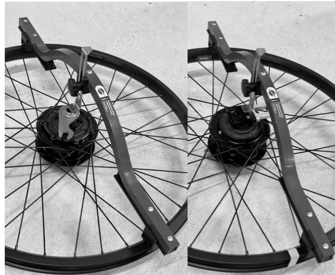
**Wheel dish:** The wheel dish can be checked by installing a hub in the SWAP cage. Remember to also install the Match cap on the non-drive side and shifter actuator on the drive side, as shown.
